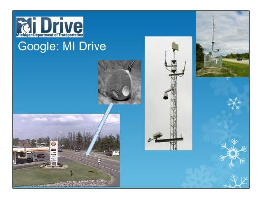
For this system to work there is tower along side the road that receives and transmits information. In some sites there are pavement sensors embedded in the road. The information from the pavement sensors is not available to the general public. At some sites there are cameras on the tower that show a real time image of the road.
