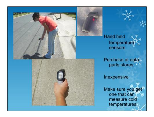
For less than \$100 you can go to most automotive stores and pick up a hand held temperature sensor. Make sure to get one that has the cold temperature range. They are used in many industries for example to measure freezer temperatures of your refrigerator or the cylinder temperature of your car.
