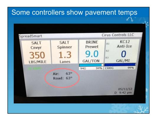
This is an example of a spreader controller that has the air and pavement temperature display built into the unit.
