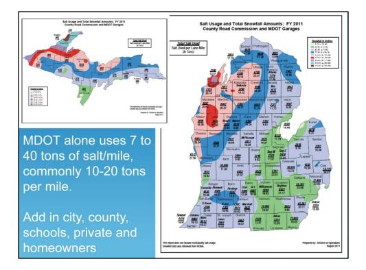
MDOT used approximately <u>526,450 tons of salt</u> and 111,750 tons of sand (statewide total) from November 2010 to May 2011 for what was a relatively heavy winter. MDOT used approximately <u>343,150 tons of salt</u> and 67,800 tons of sand (statewide total) from November 2011 through May 2012 for what amounted to a relatively light winter. (Source: MDOT Website)
