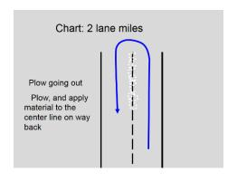
Figure 9: Suggested Plow and Apply Pattern for Deicing
