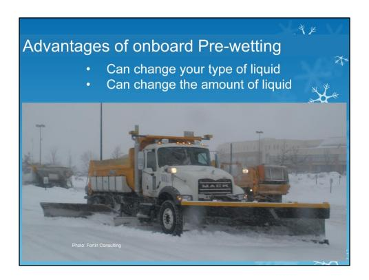
Pre-wetting salt occurs on the truck. There is a tank for liquid de-icer and a box for granular de-icer. They come together before the road although they generally are poorly mixed.
