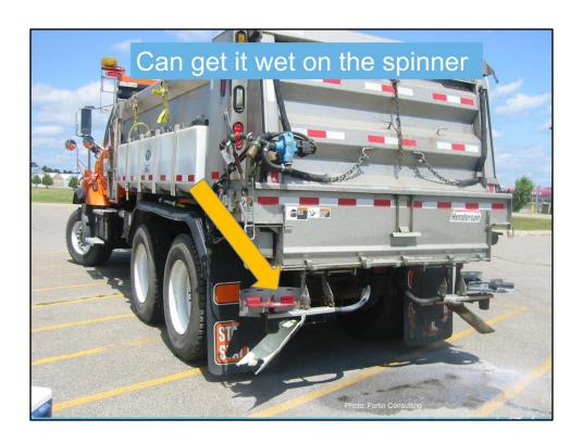
This is a very common method of pre-wetting. In this example the liquid is discharge at the spinner. It isn't perfect, Its short coming is that it is difficult to get a good blend of liquid and granular. Its advantage is it flows nicely and doesn't cause many problems.
